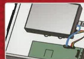
② Connect data and power cables to the motherboard and then install the cover.
